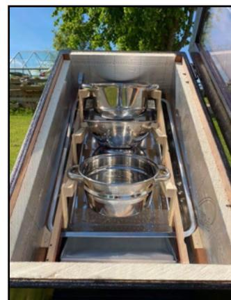
Test day: Sunday 30th May, a beautiful sunny day, I put a small amount of water in the bottom of the loaf tin to make the wax easier to remove as when cooled the wax will sit on top of the water. I then placed it in the sunshine at 9am and loaded it with dirty wax by 9:45 am the wax was starting to flow. Throughout the day and all the following day I kept adding dirty wax. The end result was just over a kilo of beautiful rendered wax.
