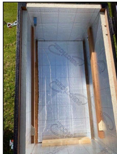
My next task was to put in a piece of 50mm x 25mm on one end to hold the loaf tin at the right angle, two side rails to hold the tray and two carrying handles at each end which also held all the insulation in place. I then needed to think about the legs, which I wanted to fold in and out to make the whole thing easier to store. After some Google research, I decided a 15 degree pitch would work, so I propped up one end of the box to 15 degrees so that I could work out the length of the legs.
